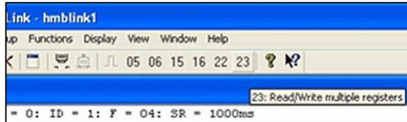
24. Double-click the top register. When the Enter Value box appears, enter the new value you want to write to this register. The following figure shows writing a value of **2**, which is the Tare command number.
