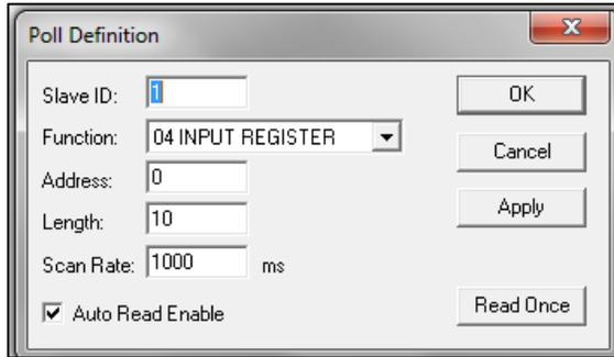
21. On the Hardy Modbus-Link page, from the **Display** menu, click **Float**. The Weight value appears in register 6 (net) or register 8 (gross). Other registers are not float values, so be aware of random numbers in other registers.
