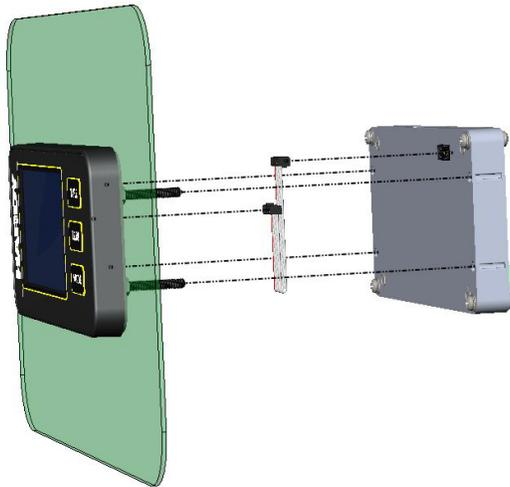
**Figure 3-4. Sliding the Instrument Half-way on to the Rods**
