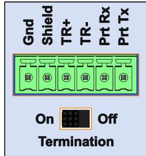
Figure 3-10. Serial Communications Terminal Block
