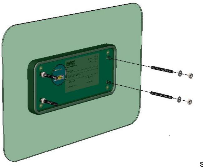
Figure 3-2. Installing Four Screw Rods into the Front Panel Display
