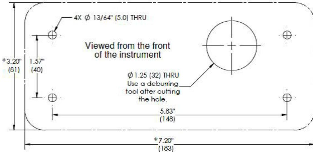
Figure 3-1. Panel Hole Dimensions (Not to Scale)
