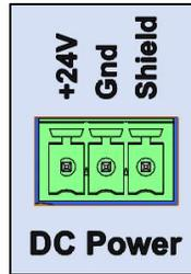
Figure 3-11. DC Input Power Terminal Block
