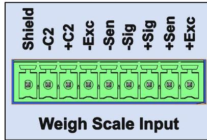
Figure 3-9. Weigh Scale Input Terminal Block
