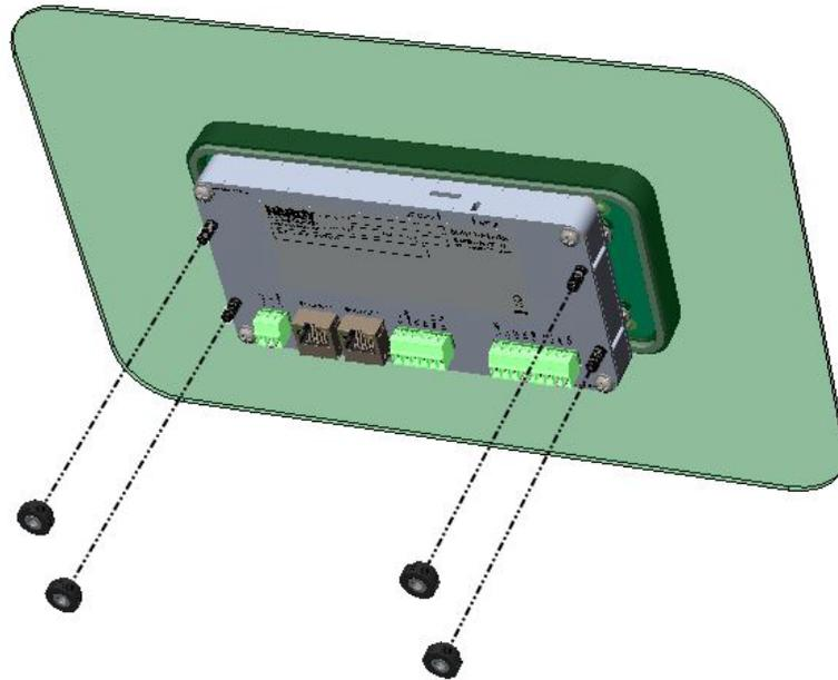
Figure 3-5. Installing and Tightening the Four Keeper Nuts
