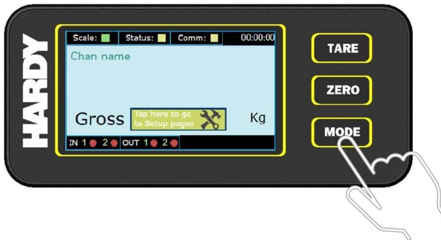
Figure 4-1. Accessing the Set-up Menus
