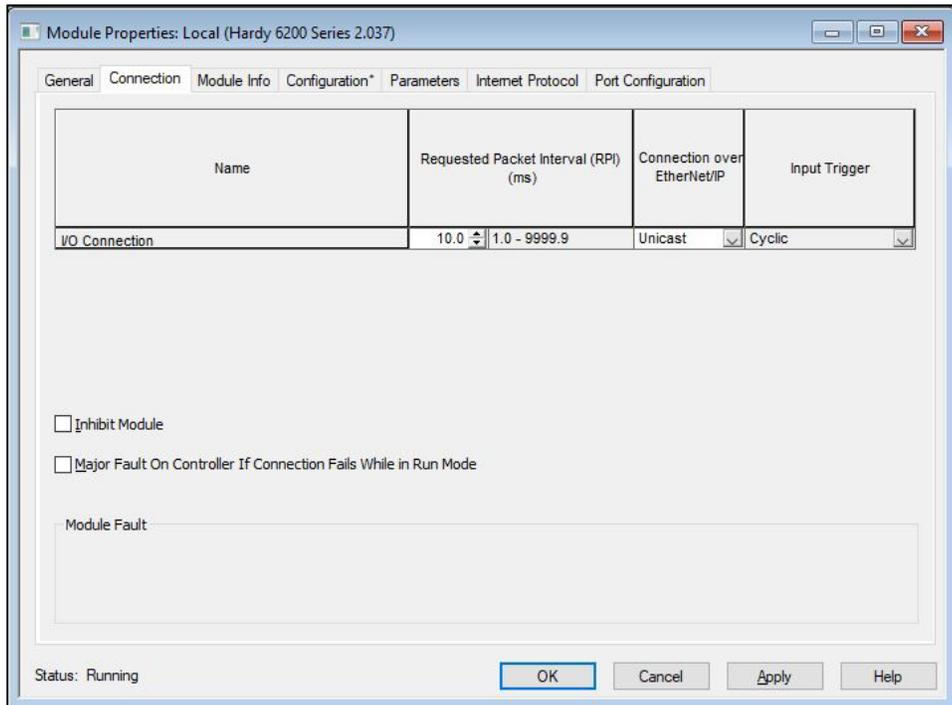
7. Click **OK**. The module appears in the controller organizer in the I/O configuration under the **Ethernet** section.
